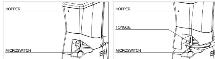
The push button that controls this device is operated by a tongue under the hopper. If the hopper is removed or not properly in place, the microswitch prevents the appliance from working. To ensure the hopper is positioned correctly it must be fixed to the casing using the relevant pins.
