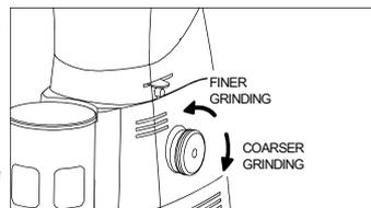
The adjustment must be performed with the motor on, and preferably without any coffee between the grinding blades. Grind small amounts of coffee in order to determine the optimal degree of fineness.
