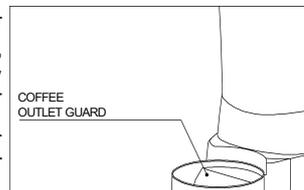
Before reconnecting the appliance to the power supply, fix the safety device to the doser, or to the funnel, by relevant screws.
