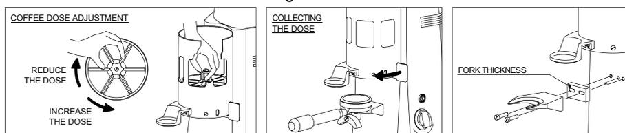
For the coffee to fall on the filter holder, the support fork can be moved sideways using the two holes that allow the best placement. If necessary, use shims (included in the package) to back the position of the fork. After finding the best position, fix the fork with the appropriate screws.
