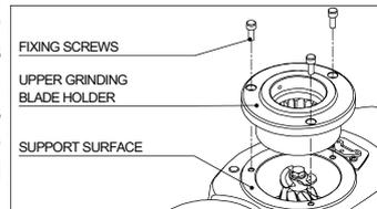
After replacing the upper grinding blade holder on the tray, tighten the screws. Refit the hopper properly.
