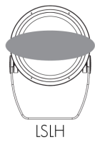
LSLH - Linear spread lens horizontal distribution
