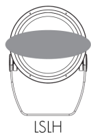
LSLH - Linear spread lens horizontal distribution
