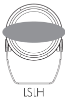
LSLH - Linear spread lens horizontal distribution
