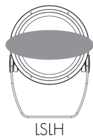
LSLH - Linear spread lens horizontal distribution
