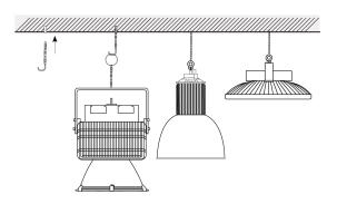
• Surface Mounted Installation: In doing wall, ceiling or seat connection, mark first the position of the screw holes on the mounting plate to the area where you will be placing the light fitting. Use an electric drill for making holes enough for screw plugs to fit in. Once done, fix the light fitting into position using appropriate metal screws. A safety chain should also be used for backup.
