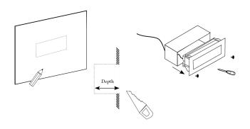
STEP 2: Screw in and fix the canister into the wall to hold it firmly in place, connect the electrical wirings to the light. You may need to use a heat shrink tube or any waterproofing connectors to prevent the wiring connection in contact with water if the application is outdoor. Again for your safety, please make sure that the supply cable power or switch has been properly turned off and no electrical voltage is present.
