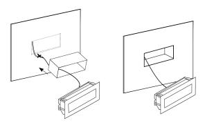
**STEP 3:** Once done, put back the light inside the canister by screwing it in or aligning the clips with the canister while gently pushing inward (Polyurethane foam sealing agent can be considered to use for permanent installation or security concern).
