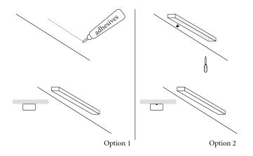
• Suspended Installation: Install the extrusion suspension cable into the ceiling first with the provided metal screws and install the other end into the extrusion, one at a time. Care must be taken with installing the screws that they are straight and fully set in place. Then adjust the length of the suspension cable as per the preferred height. Make sure that the
