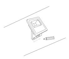
**STEP 2:** Fix the light fitting into the wall with hexagonal head metal screws using wrench. If the installation is on concrete, you need to use screw plugs or anchors.
