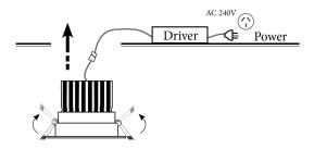
**STEP 3:** Once fully inserted, the clip shall hold perfectly the LED recessed downlight in place.
