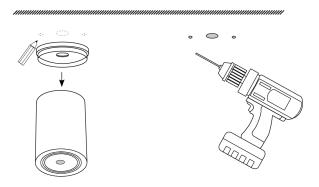
**STEP 2:** Position and install the set screw to fix the base of the light fitting into the ceiling then connect the power cables.
