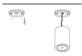
**STEP 3:** Connect the light fitting to the base by doing twist to lock. Some designs need to be screwed on the sides to interlock both.
